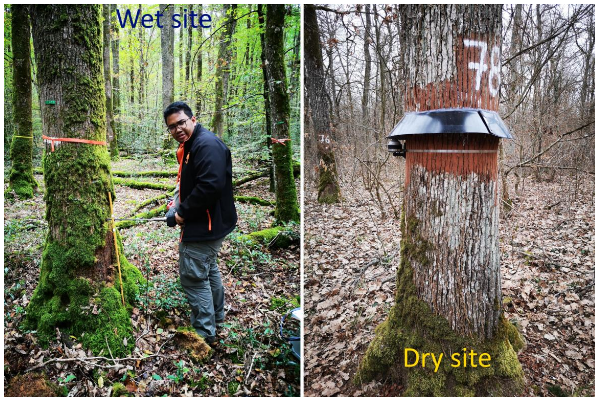
Core sampling in the wet site by Arivoara Rabarijaona (left). Automated dendrometer newly installed in the Harth site (right)
